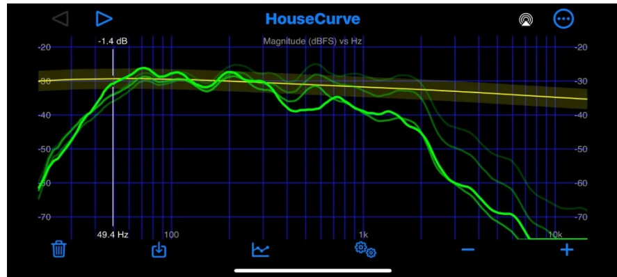
Figure 2 – The effects of slot loading on a bass driver. The various curve traces show frequency response as the area of the slot is increased and decreased. The slot acts like a 1 st order electronic filter, attenuating high frequencies (12dB at 1,100 hz for example)
